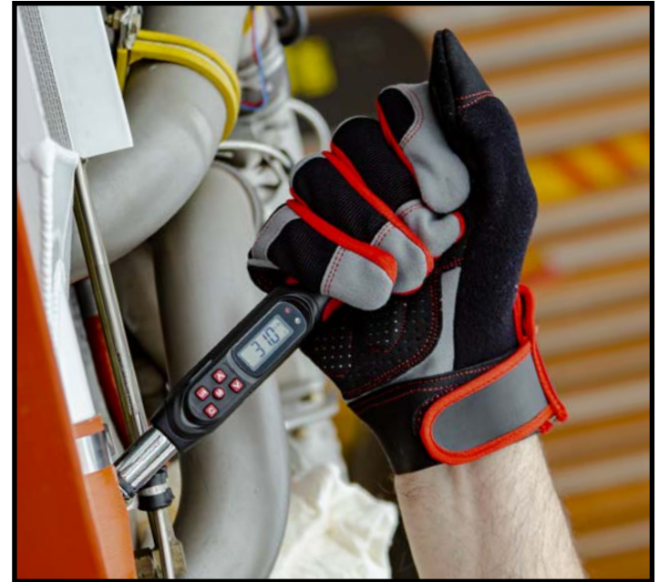
EDWM020 used to tighten motor compartment bolts on Cirrus SR22 aircraft.
