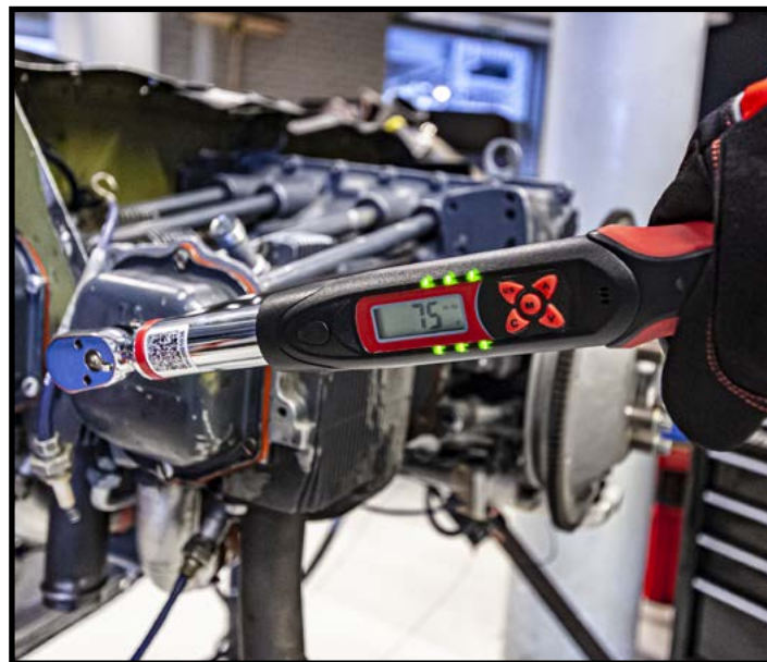
EDWS030 tighten bolts on a engine.
